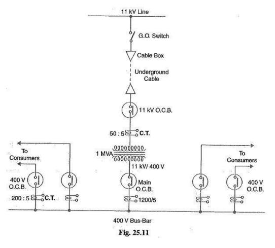
3. The secondary of transformer supplies to the bus-bars via the main O.C.B. From the bus-bars, 400 V, 3-phase, 4-wire supply is given to the various consumers via 400 V O.C.B. The voltage between any two phases is 400 V and between any phase and neutral it is 230 V. The single phase residential load is connected between any one phase and neutral whereas 3-phase, 400 V motor load is connected across 3-phase lines directly.
