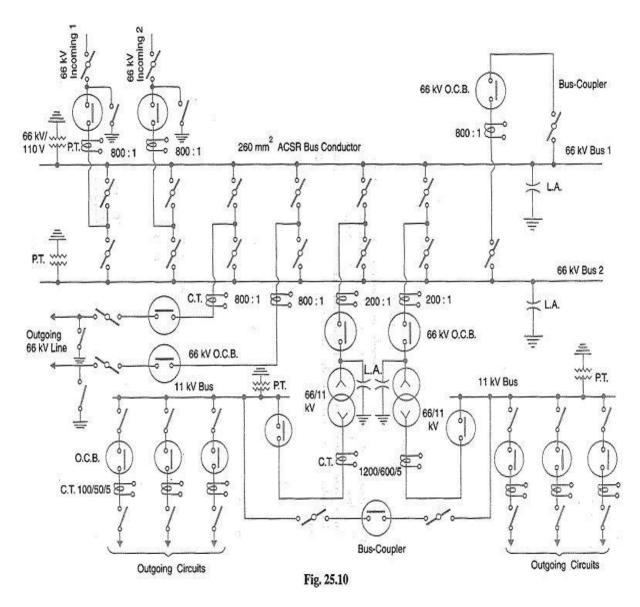
3. There is an arrangement in the sub-station by which the same 66 kV double circuit supply is going out i.e. 66 kV double circuit supply is passing through the sub-station. The outgoing 66 kV double circuit line can be made to act as incoming line.
